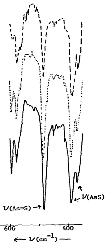
Figure 9: Temperature dependence of the infrared spectrum of (\text{CH}_3)_4\text{As}_2\text{S}_2 in carbon tetrachloride and 1,1,2,2, tetrachloroethane at 30^\circ\text{C} (—), 60^\circ\text{C} (-----) and 75^\circ\text{C} (---) 104 .
